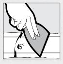
To apply drywall compound neatly, dip the knife sideways into the pan so you load only half the width of the blade.
