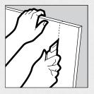
To break the panel core, securely grasp the board edges on both sides of the score line and snap board with a quick, firm movement.
