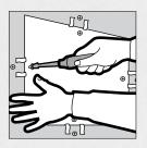
d. Remove tabs from each drywall repair clip. Apply compound and tape to all four section sides. Do not overlap tape. Apply second and third coats of drywall compound, allowing each coat to harden before applying next coat and feathering out from previous coats. Sand and prime when dry.
