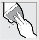
Center and lightly press tape into wet drywall compound with fingers. Draw 125 mm (5 in.) knife firmly along drywall to tightly embed tape. Be sure there is sufficient drywall compound under tape to prevent blistering of the tape.
