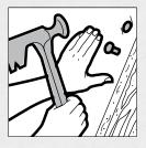
SCREW ATTACHMENT Space screws a maximum of 300 mm (12 in.) apart on ceilings, 400 mm (16 in.) on walls and at least 10 mm (3/8 in.) from ends and edges of panels. Sink screws to just below the panel surface, leaving the paper intact.
