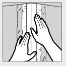
Use the knife (or a damp sponge) to remove excess compound, eliminating any air bubbles under the paper. Allow to dry.
