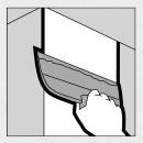
Allow third coat to dry overnight (drying time may vary, depending on temperature, humidity and jobsite conditions). Lightly sand imperfections in finished joints, corners and over fastener heads. Carefully remove sanding dust with damp sponge. Use a dust collection with a HEPA filter with power sanding. Wear a dust mask if excessive dust is produced and the area cannot be ventilated.
