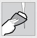
c. Embed tape in compound to bridge crack. Draw knife firmly over crack to tightly embed tape. Let compound harden.
