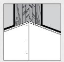
To join panels at an outside corner, lap the end of the second board over the end of the first. Make sure panels abut neatly — do not overlap or extend the end of the second board beyond the first. Fasten both panel ends to their common stud.
