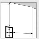
Trace the outline of the electrical box at the appropriate position on the gypsum panel.
