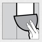
Apply drywall compound to tapered joints using a 200 mm (8 in.) knife the length of the joint.
