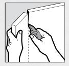
After cutting the panel, smooth the cut edge with a drywall rasp or sandpaper wrapped around a block of wood such as a piece of 50 mm (2 in.) x 100 mm (4 in.) lumber. Be sure to keep edge as square as possible. Always wear a dust mask when sanding.
