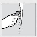
b. Apply compound to crack with 125 mm (5 in.) finishing knife.
