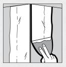
Use a 200 mm (8 in.) or larger finishing knife for outside corners (100 mm-150 mm [4 in.-6 in.]) to apply a finishing coat of the same ready-mixed or settingtype compound. Feather compound 200 mm (8 in.) from nose of trim for outside corners (25 mm [1 in.] past previous coat for inside corners). Let dry. Sand, dust and prime.
